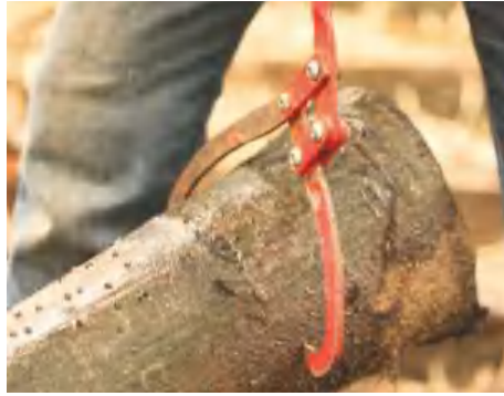
A cunning device for lifting a log. The weight makes it lock on
